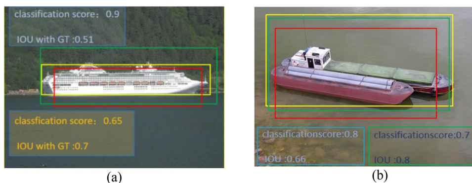
Fig. 1 The misalignment between ship classification confidence and ship localization accuracy is illustrated in the cases. The yellow bounding boxes denote the ground truth (GT), while the red and green bounding boxes are both detection results yielded by Feature Pyramid Networks (FPN) (Lin et al. 2017). As shown in picture (a), the classification score of the red bounding box is 0.65 and the green
