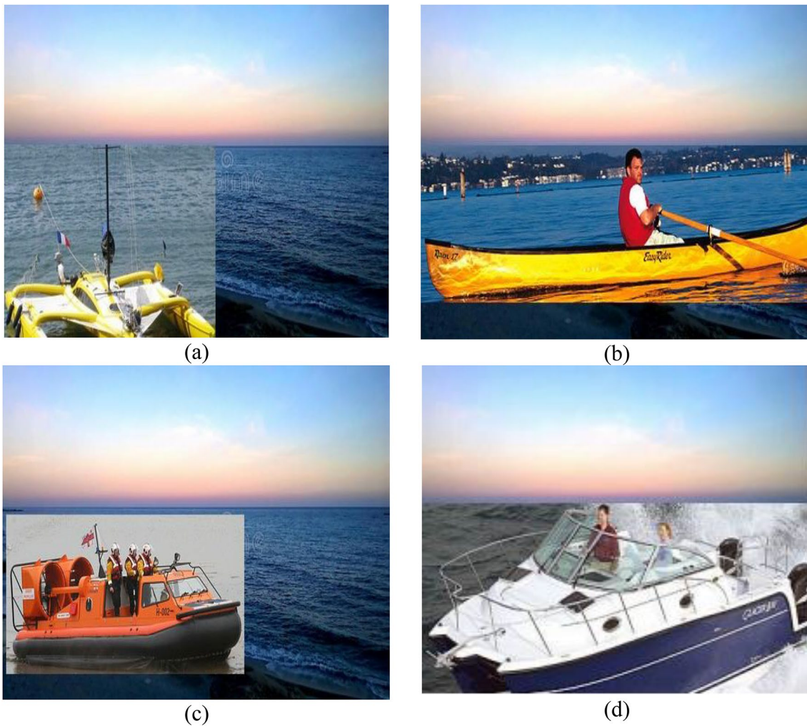
Fig. 10 Examples of the first data augmentation method to detect the sea line and then paste the ship image under the sea line. a–d are the results
