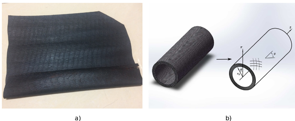
Fig. 3. Structure and parameterization of reinforcement layers.
